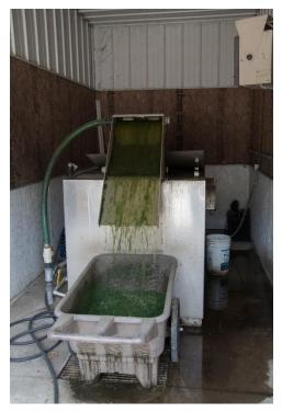
Figure 42. Clippings should be separated from washwater and managed properly to avoid water quality impacts from nitrogen and phosphorus. Photo credit: Mark Jones.
