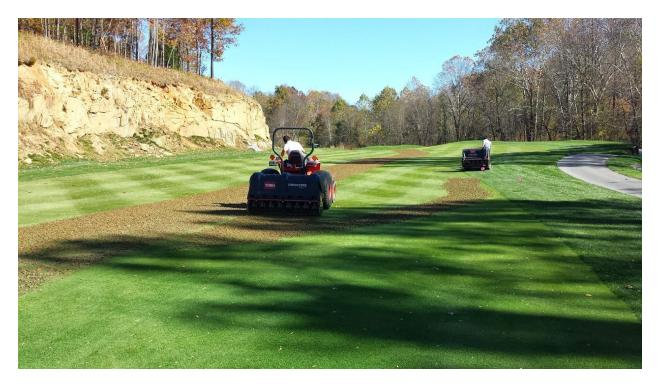
Figure 26. Aeration manages soil compaction and aids in improvement of soil drainage by removing small cores or plugs from the soil profile. Photo credit: Chris Harriman.
